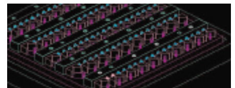
■ A multi-station fixture with spring-loaded Vs to secure different diameters (shown in dwg).
